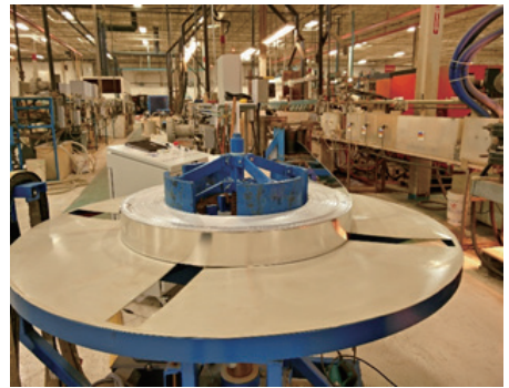
.093" material BET plated winding
